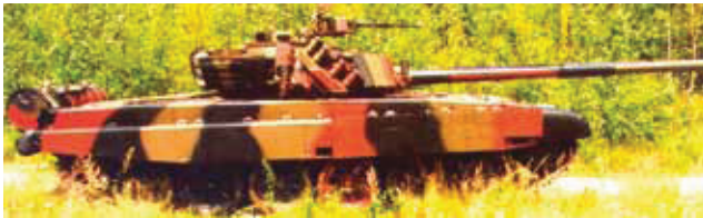
Fig. 3. Polish tank PT-91 Hard with quickly assembled blocks of ERAWA-1 and ERAWA-2 reactive cassettes (III generation)
