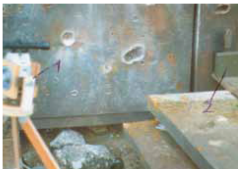
Fig. 7. Scheme of test of protective ability of ERAWA-2 cassette (2) by firing with the use of EFP warhead (1) ( d = 100 mm, h = 85 mm), ( \infty = 60^\circ )
