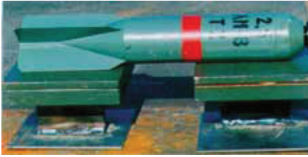
Fig. 17. Scheme of resistance test of ERAWA-1 cassette to detonation and destruction during burning of incendiary bomb ZAB-2,5 containing thermite (3000 °C) on it
