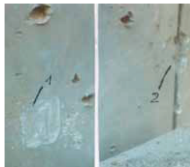
Fig. 8. Traces on RHA armour after penetration of ERAWA-2 cassette with warhead EFP; 1 - trace of detonation of ERAWA-2 cassette, 2 - trace of destroyed EFP projectile (EFP - h = 85 mm), h_w = 5 mm, protective ability of cassette CP = 94\% , ( \infty = 60^\circ )
