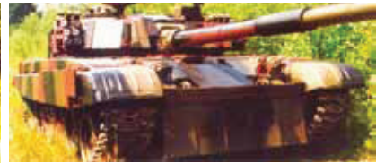
Fig. 3. Polish tank PT-91 Hard with quickly assembled blocks of ERAWA-1 and ERAWA-2 reactive cassettes (III generation)
