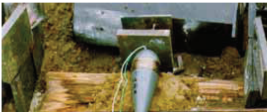
Fig. 11. Scheme of resistance test of ERAWA-1 cassettes to detonation and destruction with explosion of 82 mm mortar grenade
