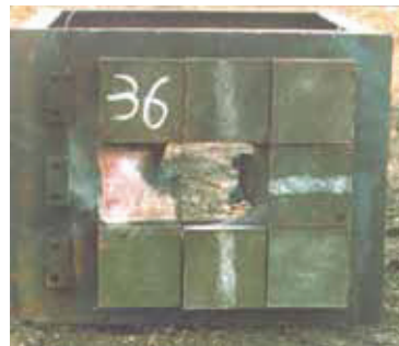
Fig. 5. Detonated ERAWA-1 cassette and destroyed neighbouring cassettes of block of nine cassettes, with 125 mm projectile BK-14M (HEAT, \infty = 60^\circ ). Penetration of RHA armour h_w = 30 mm, protective ability of cassette CP = 94\%
