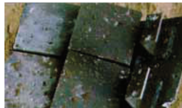
Fig. 12. ERAWA-1 cassettes after explosion of 82 mm mortar grenade
