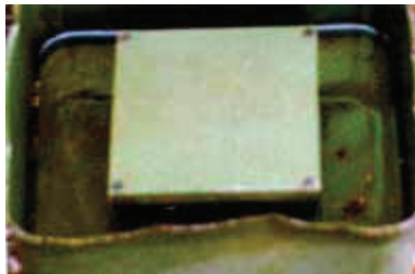
Fig. 13. Scheme of resistance test of ERAWA-1 cassette to detonation and destruction during burning of petrol around it
