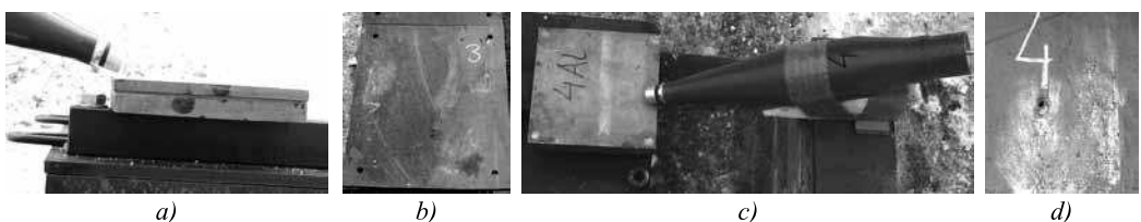
Fig. 8. Panels with ERAWA-1 cassettes from aluminium alloy before and after the initiation of the PG-7 projectile at an angles of \alpha from normal to the cassette: a) panel 3, \alpha=72^\circ ; b) DP=4.5 mm and copper trace on witness plate 2 (panel 3); c) panel 4, \alpha=60^\circ ; d) DP=8 mm perforation of witness plate 2 (panel 4).
