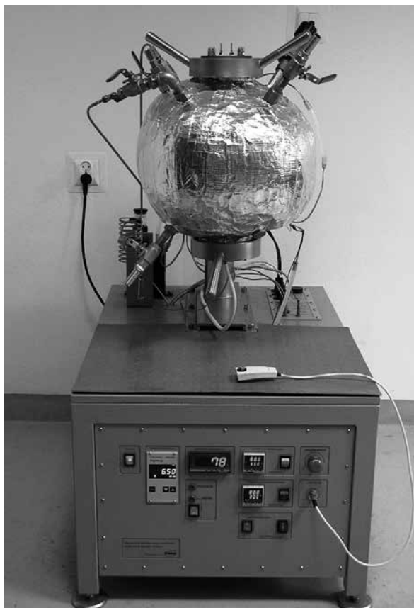
Figure 1. Test stand for determining the explosion parameters of gases and vapours.
