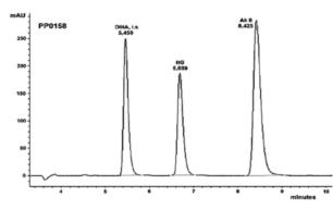
Figure 1. Chromatogram of NG and Ak II determination in the PP0158 sample.
