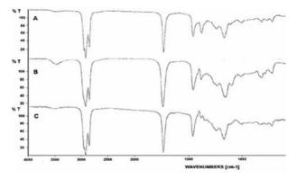
**Figure 2.** The IR spectrum of pure oils; A – lankroflex ED6, B – lankroflex L, C – lankroflex E2307.
