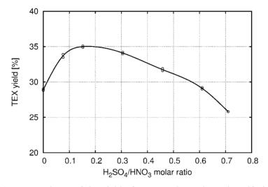
**Figure 4.** Dependence of the yield of TEX on the molar ratio sulfuric acid/ nitric acid (for DFTHP/HNO<sub>3</sub> constant ratio 33.6).
