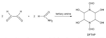
**Figure 2.** Scheme of DFTHP synthesis from formamide and glyoxal in the presence of tertiary amine.
