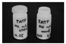
**Figure 1.** Ageing of the TATP samples was carried out in small plastic bottles (volume 20 ml, mouth diameter 17 mm, one being covered with a lid, and the other uncovered).
