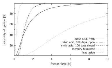
**Figure 7.** Friction sensitivity of fresh and aged TATP prepared by using nitric acid in comparison to mercury fulminate (right dotted curve) and lead azide (left dotted curve).
