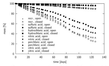
**Figure 4.** Influence on the mass loss of TATP of the acid used for TATP preparation (measured at laboratory temperature for 126 days). The lower lines are for TATP samples aged in open bottles; the upper lines are for closed bottles. The mass loss of the samples prepared using sulphuric or perchloric acid is significantly higher.
