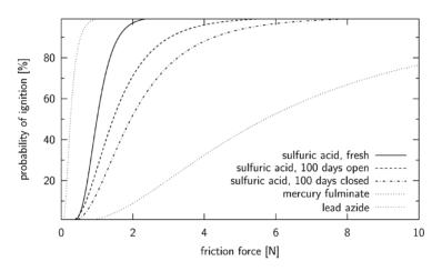
**Figure 8.** Friction sensitivity of fresh and aged TATP prepared by using sulphuric acid in comparison to mercury fulminate (right dotted curve) and lead azide (left dotted curve).
