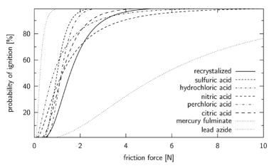
**Figure 5.** Friction sensitivity of freshly prepared TATP samples using various acids in comparison to re-crystallized TATP, mercury fulminate (right dotted curve) and lead azide (left dotted curve).
