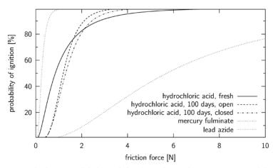
**Figure 6.** Friction sensitivity of fresh and aged TATP prepared by using hydrochloric acid in comparison to mercury fulminate (right dotted curve) and lead azide (left dotted curve).
