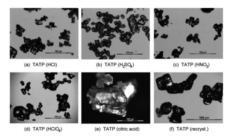
Figure 3. The crystal size and shape of aged TATP samples.
