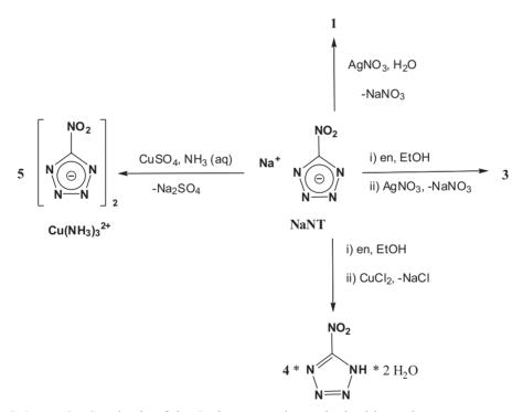
Scheme 2. Synthesis of the 5-nitrotetrazolate salts in this study.
