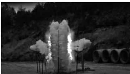
(a) The cylindrical charge of L/D = 8.3 showing symmetry and a large effect on the centreline
