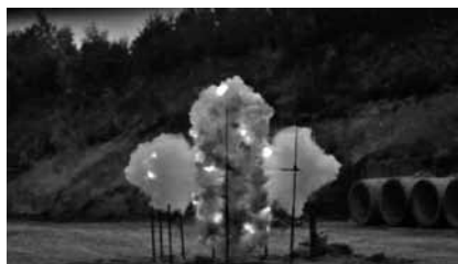
(b) The cylindrical charge of L/D = 1 , showing symmetry and larger effect on the axis
