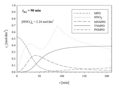
Figure 13. Variation of the reactant concentrations in the process of MPD nitration in the case of dosage of nitric acid during 90 min.
