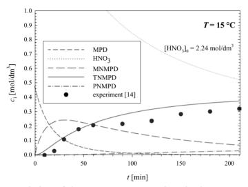
**Figure 8.** Variation of the reactant concentrations in the process of MPD nitration at 15 °C under the conditions given in [14].
