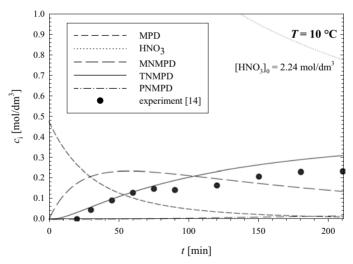
**Figure 7.** Variation of the reactant concentrations in the process of MPD nitration at 10 °C under the conditions given in [14].
