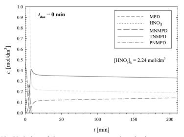
Figure 10. Variation of the reactant concentrations in the process of MPD nitration in the case of dosage of nitric acid at t = 0 min.
