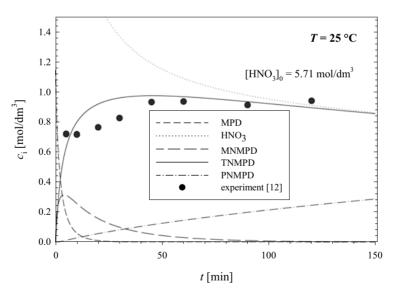
**Figure 5.** Variation of the reactant concentrations in the process of MPD nitration at 25 °C under the conditions given in [12].
