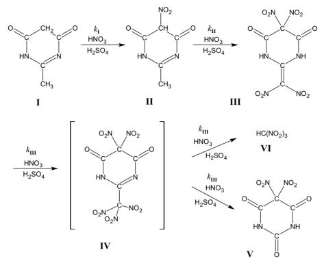
Figure 2. A scheme of MPD nitration [13].
