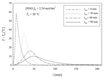
Figure 14. Variation of the temperature of the reactants in the process of nitration of MPD for various nitric acid addition times.
