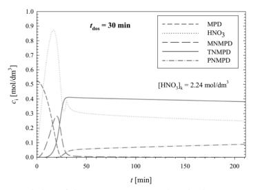
Figure 11. Variation of the reactant concentrations in the process of MPD nitration in the case of dosage of nitric acid during 30 min.
