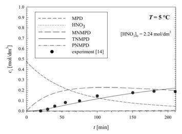
**Figure 6.** Variation of the reactant concentrations in the process of MPD nitration at 5 °C under the conditions given in [14].
