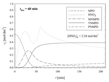
Figure 12. Variation of the reactant concentrations in the process of MPD nitration in the case of dosage of nitric acid during 60 min.
