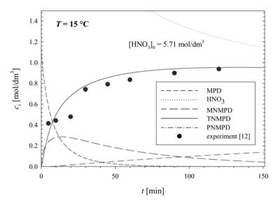
**Figure 4.** Variation of the reactant concentrations in the process of MPD nitration at 15 °C under the conditions given in [12].
