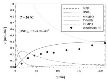
**Figure 9.** Variation of the reactant concentrations in the process of MPD nitration at 20 °C under the conditions given in [14].
