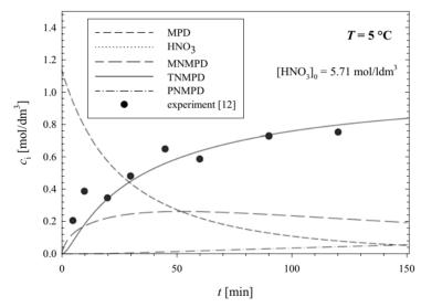
**Figure 3.** Variation of the reactant concentrations in the process of MPD nitration at 5 °C under the conditions given in [12].
