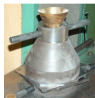
Figure 8. Mould 1 prepared for filling with the explosive.
