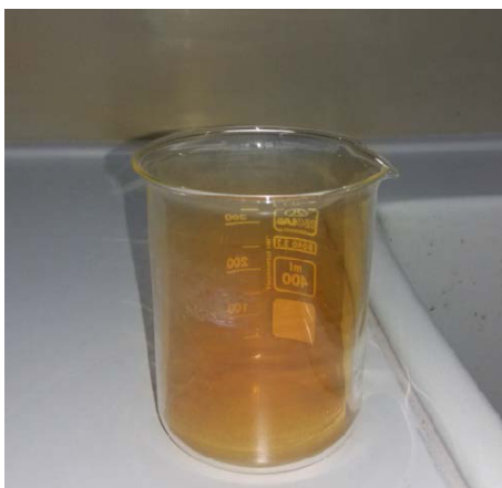
Figure 1. Nitrogen tetroxide in equilibrium with nitrogen dioxide vapour at room temperature
