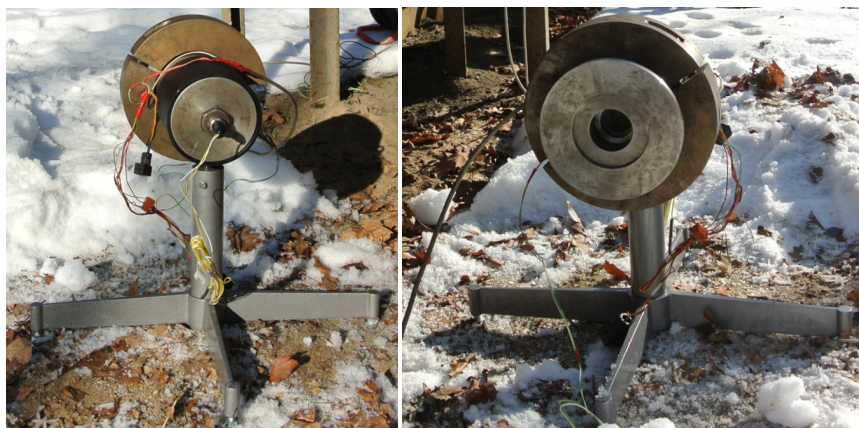
Figure 1. Modified laboratory rocket motor for investigation of gas fracturing of rocks
