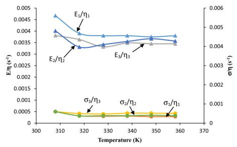
Figure 6. Variation of  $E/\eta$  and  $\sigma/\eta$  for Type-I, II and III propellants with temperature
