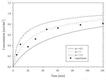
Figure 6. The concentrations of TNMPD obtained from modelling and experiment under the conditions given in [4] for a temperature inside the reactor equal to  $5 \,^{\circ}C$
