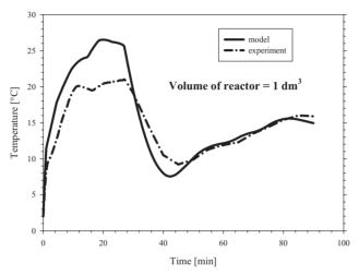
Figure 12. Temperature variation obtained from modelling with the kinetics parameters and reaction heat from [4], and the experimental variations for the 1 dm<sup>3</sup> reactor
