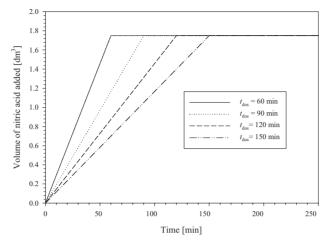
**Figure 14.** Volume variation of the nitric acid added to the reactor of volume 10 dm<sup>3</sup>
