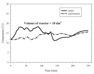
Figure 13. Temperature variation obtained from modelling with the kinetics parameters and reaction heat from [4], and the experimental variations for the 10 dm<sup>3</sup> reactor
