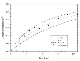
Figure 3. The concentrations of TNMPD obtained from modelling and experiment under the conditions given in [5] for a temperature inside the reactor equal to  $10 \,^{\circ}\text{C}$
