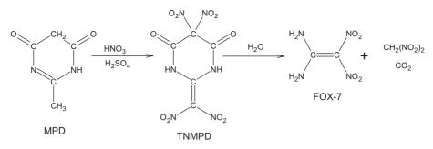
Figure 1. Scheme for the synthesis of FOX-7 [4, 5]
