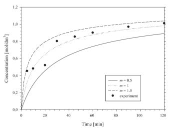
Figure 7. The concentrations of TNMPD obtained from modelling and experiment under the conditions given in [4] for a temperature inside the reactor equal to  $15 \,^{\circ}\text{C}$
