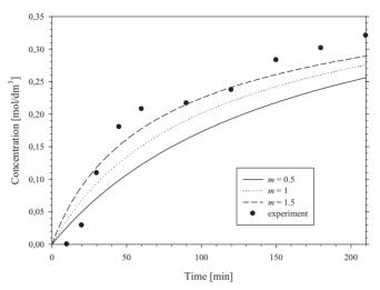
Figure 4. The concentrations of TNMPD obtained from modelling and experiment under the conditions given in [5] for a temperature inside the reactor equal to  $15 \,^{\circ}\text{C}$
