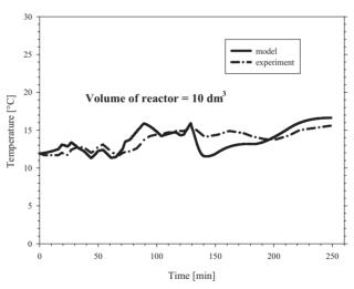
Figure 11. Temperature variation obtained from modelling with the kinetics parameters and reaction heat from [5] and [6], and the experimental variations for the 10 dm<sup>3</sup> reactor
