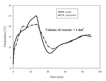
Figure 10. Temperature variation obtained from modelling with the kinetics parameters and reaction heat from [5] and [6], and the experimental variations for the 1 dm<sup>3</sup> reactor
