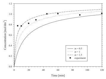
Figure 8. The concentrations of TNMPD obtained from modelling and experiment under the conditions given in [4] for a temperature inside the reactor equal to  $25 \,^{\circ}\text{C}$
