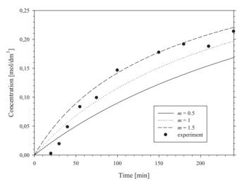
Figure 2. The concentrations of TNMPD obtained from modelling and experiment under the conditions given in [5] for a temperature inside the reactor equal to  $5 \,^{\circ}\text{C}$
