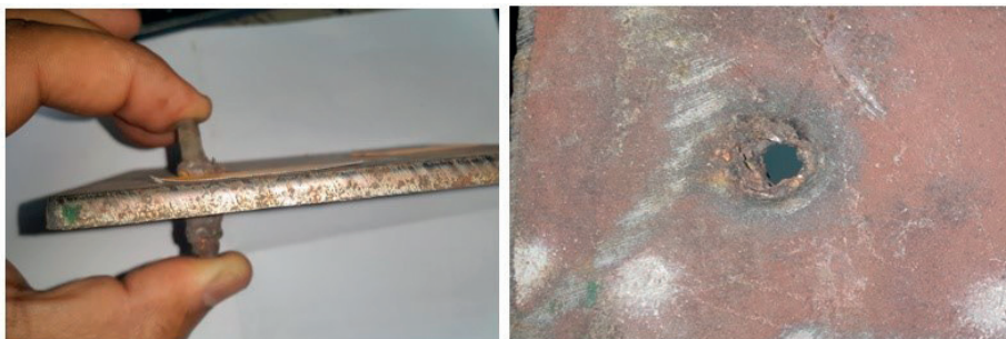
Figure 10. The first top perforated RHA plate for both copper liner (left) and powder non clogged hole (right)
