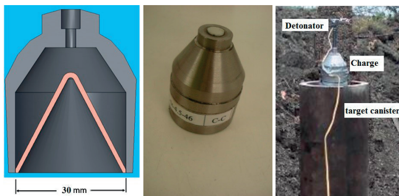
Figure 3. Test setup and the manufactured shaped charges
