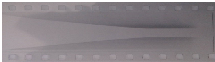
Figure 6. Typical photograph of the cylinder expansion process recorded by a high speed streak camera
