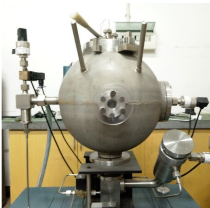
Figure 3. 20L explosion vessel experimental device
