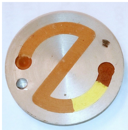
Figure 1. Unconfined (uncovered), curved, segmented pyrotechnic path pressed into the groove of the steel disc of a self-destroying timing assembly of an anti-aircraft short range missile
