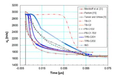
**Figure 6.** Calculated particle velocity of NM *vs.* time, obtained by different reaction rate models
