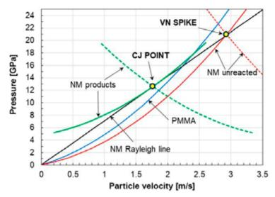
**Figure 3.** Cross plot of Hugoniots of unreacted NM and its detonation products, Rayleigh line for NM, and Hugoniot of PMMA [10]
