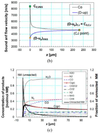
Figure 8. Spatial distribution of pressure and temperature (a), sound and flow velocity (b), and concentration of products within first 100 μm ns (25) behind the shock (c); calculation done using PB-C1.7D2 rate model
