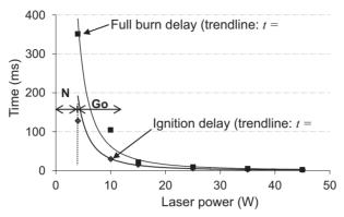
**Figure 6.** Ignition delay and full burn delay for laser ignition of HNS IV sensitized with the dye.
