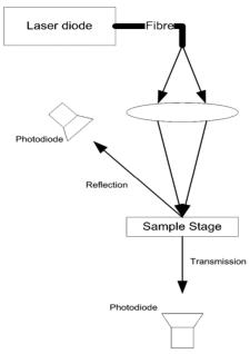
Figure 2. Experimental arrangement for the optical absorption measurement.
