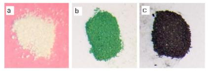
**Figure 1.** Photos of (a) HNS IV powder, and the mixtures (b) with the dye, and (c) with carbon black.
