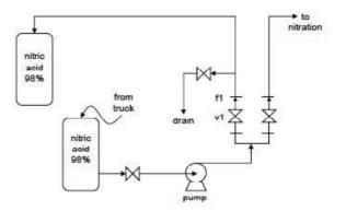
Figure 9. Nitric acid storage facility
