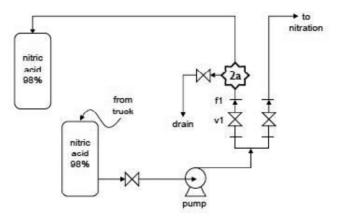
Figure 10. Selected hazard in nitric acid storage facility
