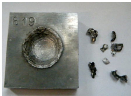
Figure 11. Plate dent and fragments after explosion.
