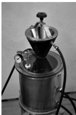
Figure 4. Arrangement for filling the mould with the propellant slurry.
