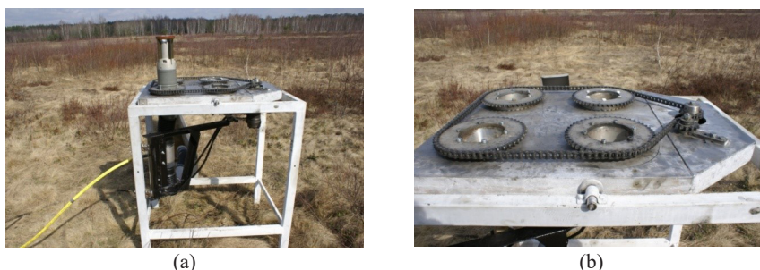
Figure 1. Details of the device used for washing out explosive materials: (a) general view of the 125 mm bullet inserted into the working socket; (b) four-socket module working table
