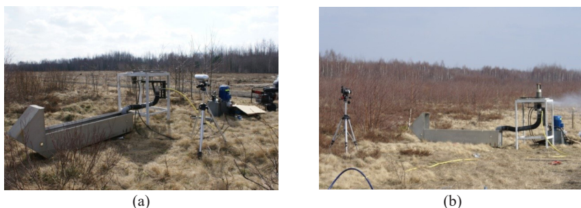
Figure 2. General view of the universal test stand: (a) location of the individual components; (b) process of washing out TNT from a 125 mm shell
