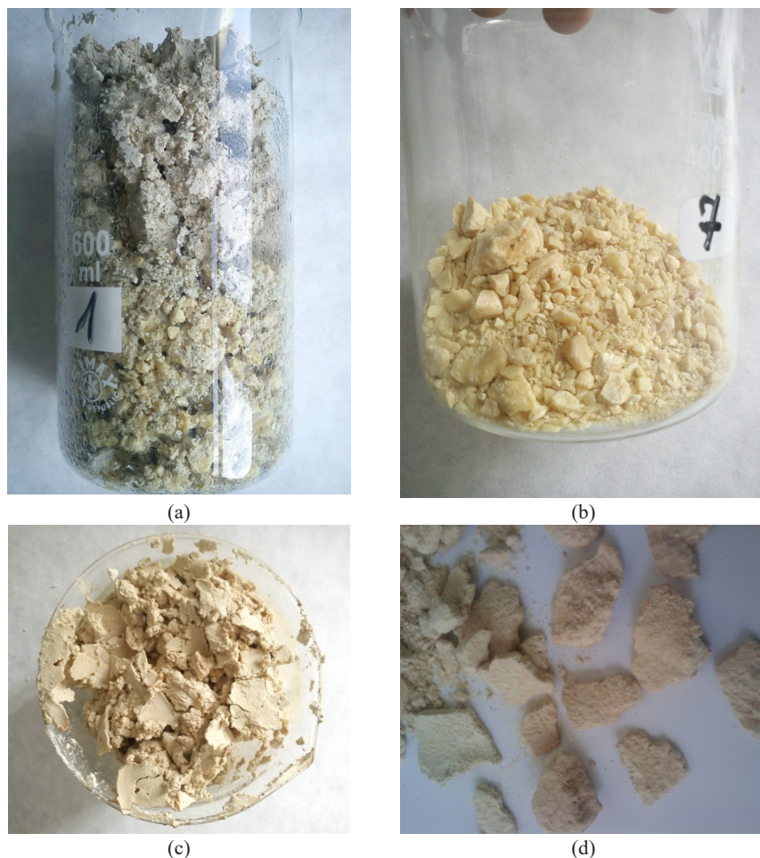
Figure 9. Differentiation in the structure of the TNT particles washed out using a high-pressure water jet: (a) mixture of granules from the finest particles (dried “foam”) and crumbs of “semolina” stuck together; (b) dry grains of “semolina”; (c) the finest particles, from dried “foam”, stuck together; (d) particles formed from melted TNT
