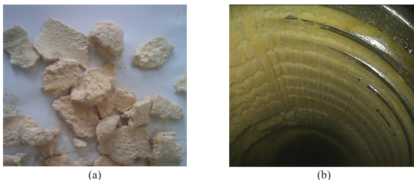
Figure 12. Collected particles of molten TNT: (a) formed during washing out with a water jet at a pressure of 260 MPa and its labels; (b) 100 mm shells remaining in the furrows of the thread in the igniter hole
