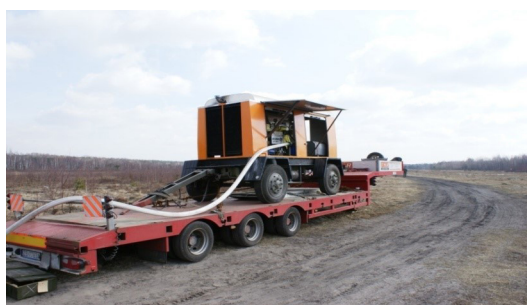
Figure 3. Hammelmann's high pressure hydraulic monitor HDP 164 ( p_{\max} = 300 MPa, Q_{\max} = 0.5 dm 3 ·s -1 )
