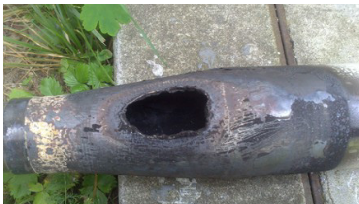
Figure 1. The effect of the metal body of the rocket motor being burnt through
