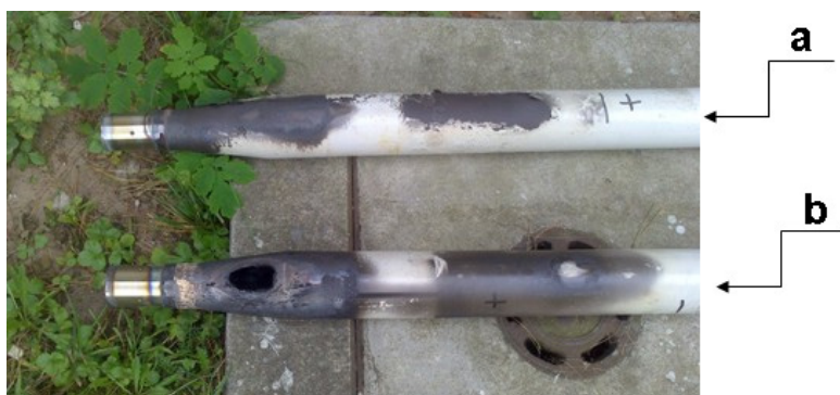
Figure 2. Rocket motor bodies after static ballistic test: a) with modernized thermal insulation, b) with extant thermal insulation
