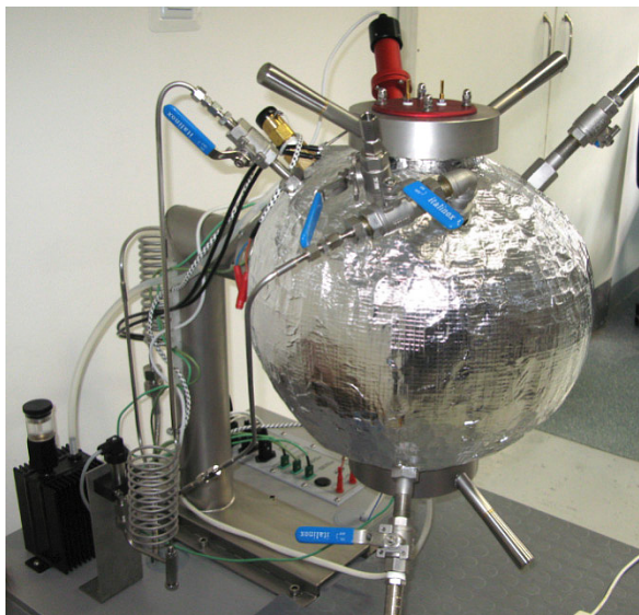
Figure 1. Test tank for determining the explosive parameters of gases and liquid vapours
