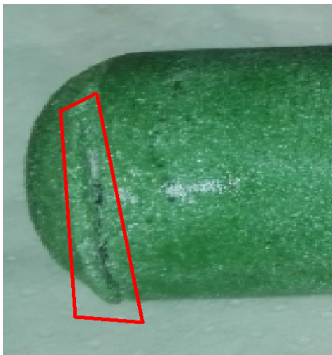
Figure 3. Inhibitor damage in the upper part of the charge
