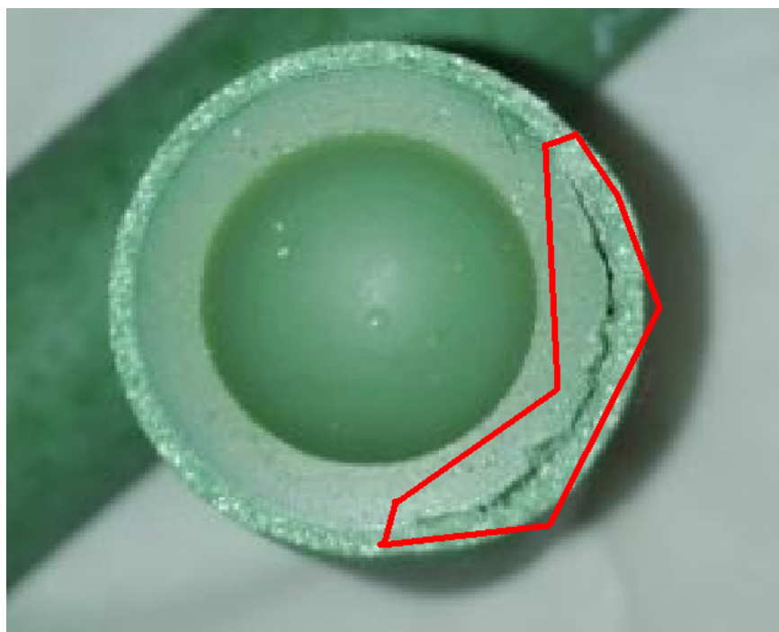
Figure 4. Inhibitor damage in the lower part of the charge
