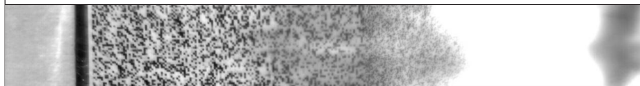
Photograph 2. (Through \Delta t \approx 333 \mu s after Photograph 1) – ignition of the EC-2 formulation and initiation of detonation in the cord has occurred – a powerful flash of light is visible due to the output of the products of explosion.
