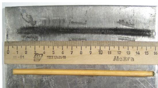
Figure 14. View of the witness plate after initiation of cord DShE-12.
