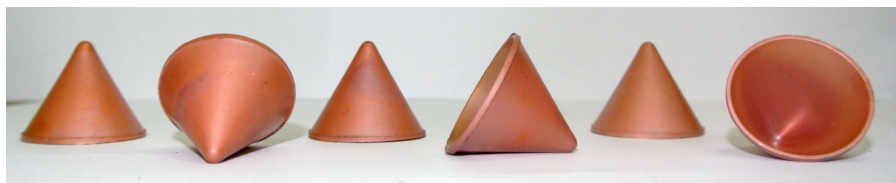
Figure 2. Liners made from copper (ECu) powder.
