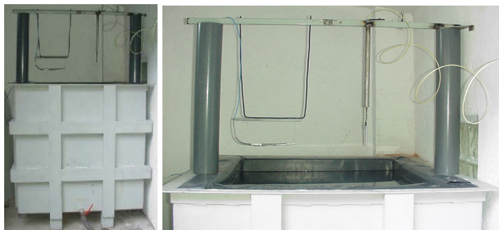
Figure 6. The arrangement for the underwater explosion tests (left) and the positioning system with the sensor and detonator (right).
