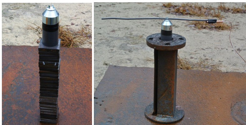
Figure 4. The test arrangement for firing the shaped charge: view of the shaped charge filled with TKX-55 placed at the standoff distance on the stack of witness plates (left) and the complete arrangement for the test (right).
