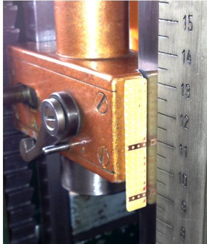
Figure 2. Reflector strip attached to the drop weight.
