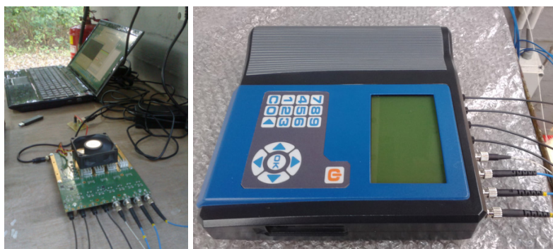
Figure 1. OPTIMEX 4+4 system during outdoor trials (left) and final prototype of the handheld 4+4 version (right) complemented with a graphical display and keyboard as a user interface
