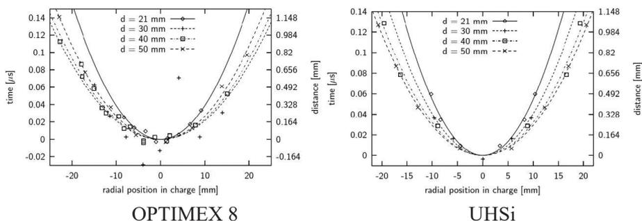
**Figure 10.** Influence of charge diameter on the detonation front curvature for  $L/D=4$ . Data from the OPTIMEX system were evaluated with the threshold set 5% below saturation.
