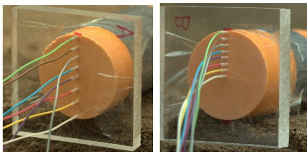
**Figure 3.** The two charge arrangements with fibers either spaced out along the entire diameter (left) or only along the radius, from the charge centre to its edge (right).
