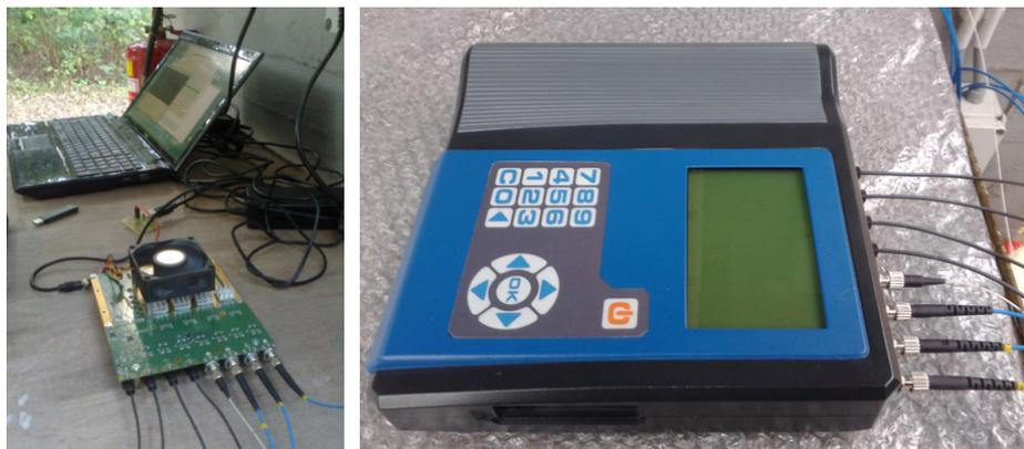
**Figure 4.** OPTIMEX 4 + 4 system during outdoor trials (left) and the final prototype of a handheld 4 + 4 version complemented with a graphical display and keyboard as a user interface (right).
