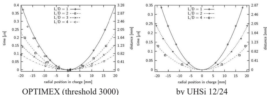
**Figure 11.** Experimentally determined detonation front curvatures as a function of length to diameter ratio for a 40 mm diameter charge.
