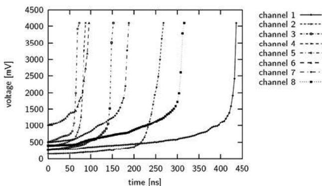
**Figure 8.** Intensity of light acquired by the fiber probes as a function of time. 4096 is a bit depth (12 bit) and on this diagram represents the cut-off value.
