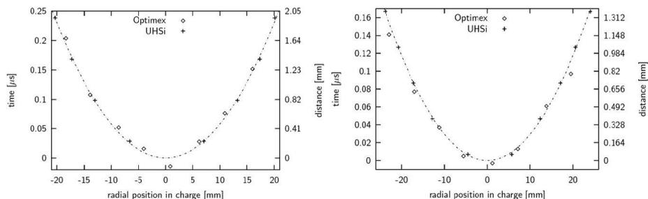
**Figure 12.** Comparison of detonation front curvatures measured by an 8 channel OPTIMEX and UHSi, diameter 40 mm,  $L/D = 2$  (left) and  $L/D = 4$  (right).
