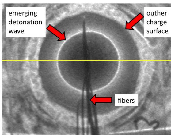
**Figure 6.** Example of a UHSi frame showing the position of the detonation front, charge outer surface and the OPTIMEX fibers (exposure 25 ns).
