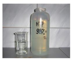
Fig. 2. A sample of 98%+ HTP to be used for rocket propulsion experiment
