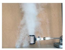
Fig. 3. Decomposition of a sample of HTP caused by potassium permanganate
