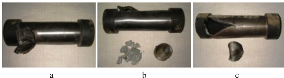
Figure 8. The tubes after parallel shots for (a) CompNTO, (b) CompNTOR and (c) cast TNT.
