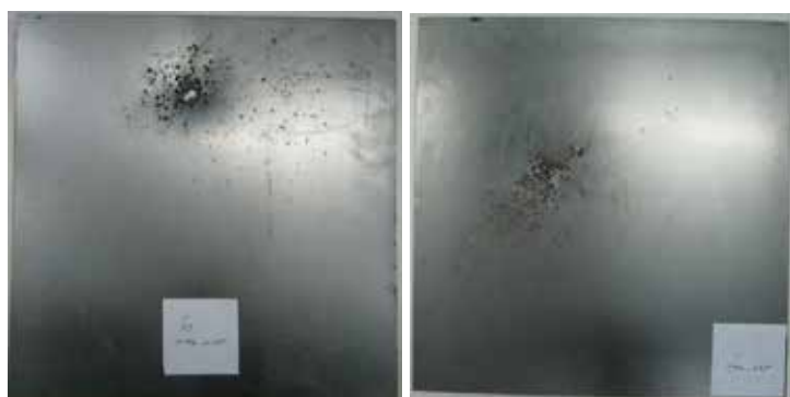
Figure 3. Witness plates hit by particles of jets striking the reactive armour at 60° and 30° (NCC20+S composite of a thickness of 9 mm).
