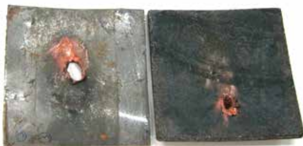
Figure 2. Upper and lower steel plates after hitting by the cumulated jet at an angle of 30^\circ (NCC20+S composite, h = 18 mm).
