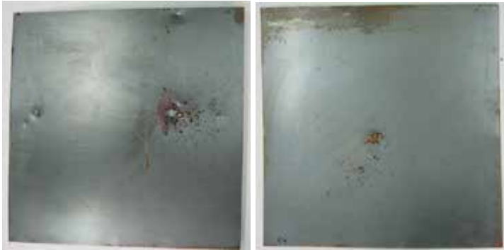
Figure 4. Witness plates hit by particles of jets striking the reactive armour at 60° and 30° (NCC20+S composite of a thickness of 18 mm).
