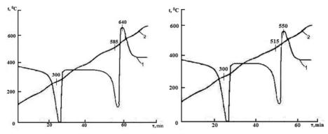
Figure 1. Thermograms of the decomposition of neat PP (left) and PP containing 3 wt.% copper(II) oxide (right). The DTA and temperature curves are labelled as curves 1 and 2 respectively
