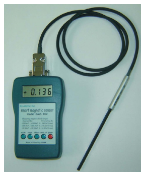
Figure 4. SMS-102 magnetic field meter.
