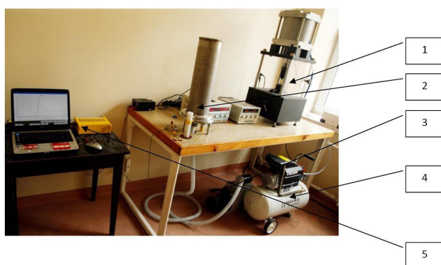
Figure 3. Experimental setup – general view. 1 – press for preparation of tablets, 2 – test chamber, 3 – vacuum pump, 4 – air compressor, 5 – data acquisition system.
