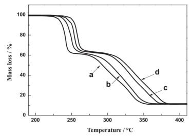
Figure 3. TG curves of HNIW/AP (1:1) at heating rates of 5 °C·min<sup>-1</sup> (a),  $10 \text{ °C·min}^{-1}$  (b), 15 °C·min<sup>-1</sup> (c) and 20 °C·min<sup>-1</sup> (d).
