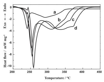
Figure 4. DSC curves of HNIW/AP (1:1) at heating rates of 5 °C·min<sup>-1</sup> (a),  $10 \text{ °C·min}^{-1}$  (b), 15 °C·min<sup>-1</sup> (c) and 20 °C·min<sup>-1</sup> (d).
