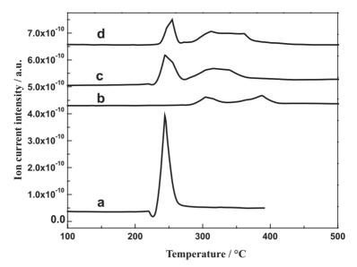
Figure 5. MS of m/z 18 of HNIW (a), AP (b), HNIW/AP (1:1) (c) and HNIW/AP (1:2) (d) at a heating rate of  $10 \degree C \cdot min^{-1}$ .
