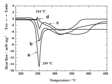
**Figure 2.** DSC curves of HNIW (a), HNIW/AP (1:1) (b), HNIW/AP (1:2) (c) and AP (d) at heating rate of 10 °C · min<sup>-1</sup>.
