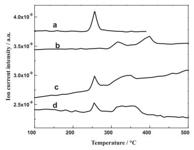
Figure 6. MS of m/z 44 of HNIW (a), AP (b), HNIW/AP (1:1) (c) and HNIW/AP (1:2) (d) at a heating rate of 10  $^{\circ}C \cdot min^{-1}$ .
