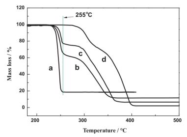
Figure 1. TG curves of HNIW (a), HNIW/AP (1:1) (b), HNIW/AP (1:2) (c) and AP (d) at heating rate of  $10 \degree C \cdot min^{-1}$ .
