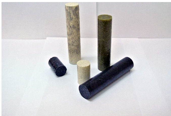
Figure 6. Examples of propellant mouldings prepared for testing in laboratory motors
