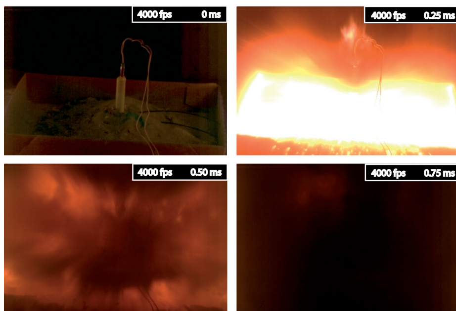
Figure 10. Detonation velocity measurement of NG-N1 (4000 fps, 4 frames).
