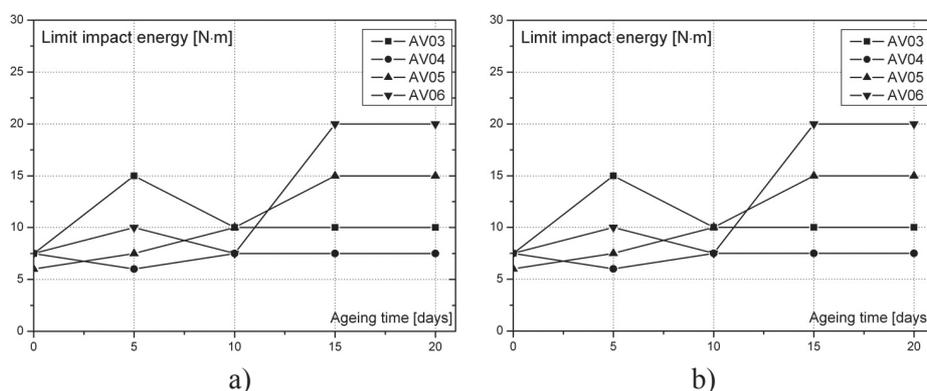
**Figure 7.** a) Ageing behaviour of the impact sensitivity expressed as the limit impact energy values according to BAM method; b) Ageing behaviour of the friction sensitivity expressed as the limit friction force values according to BAM method.
