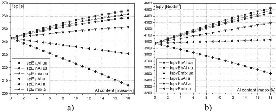
**Figure 1.** a) Gravimetric impulse  $I_{sp}$  vs. solid filler of formulations containing aged and unaged aluminium powder; b) Volumetric impulse  $I_{spv}$  vs. solid filler of formulations containing aged and unaged aluminium powder.
