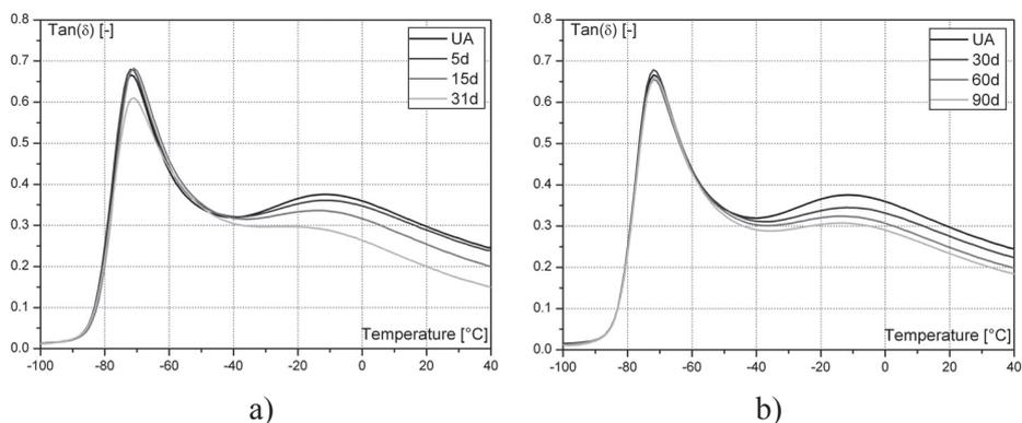
**Figure 6.** a) Loss factor vs. Temperature for the propellant AV04 aged at 90 °C; b) Loss factor vs. Temperature for the propellant AV04 aged at 70 °C.
