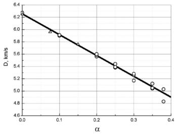
**Figure 3.** Detonation velocity D for NM/M mixtures with various methanol weight content of  $\alpha$ :  $\circ$  – present work data;  $\Delta$  – from Ref. [7].
