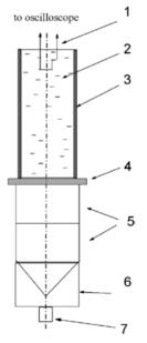
Figure 1. Experimental assembly scheme: 1 – stepped electromagnetic gage; 2 – liquid under study; 3 – confinement; 4 – plexiglass layer; 5 – explosive (pressed TNT); 6 – explosive lens; 7 – tablet for electric detonator.
