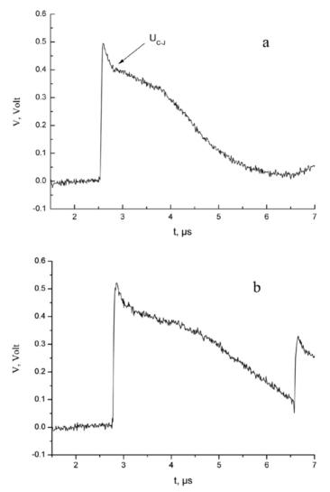
**Figure 2.** Oscillograms of particle velocity profiles U(t) for 70/30 NM/M mixture: a – gage made of 30 micron thick aluminum foil; b – stepped gage, 50 micron thick.
