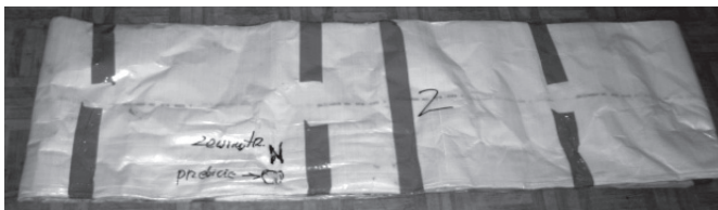
Figure 15. A view of destruction of cushion layer of cylinder cover version II.
