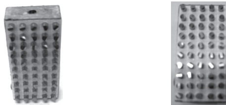
Figure 3. TNT slab 100x50 mm with 100 pcs of standard fragments placed on two sides.
