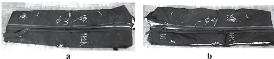
Figure 21. View of outer side of cylinder where the (a) 3 mm and (b) 4 mm bearing balls operated.
