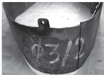
Figure 20. View no. 2 of outer side of metal sheet after (a) 3 mm and (b) 4 mm fragments hits.
