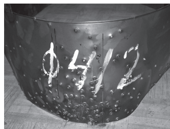
Figure 20. View no. 2 of outer side of metal sheet after (a) 3 mm and (b) 4 mm fragments hits.
