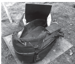
Figure 19. Post-explosion view of destruction of cylinder fibrous cover version III and screens after the explosion: a – cylinder fibrous cover version III; b – fabric screens.
