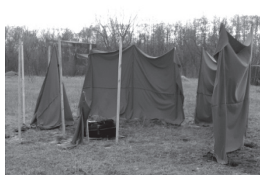
Figure 19. Post-explosion view of destruction of cylinder fibrous cover version III and screens after the explosion: a – cylinder fibrous cover version III; b – fabric screens.
