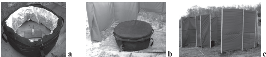
Figure 8. Cylinder fibrous cover version I, view before explosion: a – with TNT slab and balls, without lid; b – with the lid put; c – surrounded with screens of a fabric.
