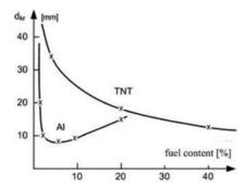
Figure 1. Dependence of critical diameter of AN mixtures vs. a fuel content.
