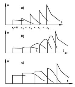
**Figure 2.** Profiles of a mass velocity during development of detonation in heterogeneous explosives [11]; TNT of density 0.9 g/cm<sup>3</sup> (a), pressed TNT of density 1.6 g/cm<sup>3</sup> (b), casted TNT of density 1.6 g/cm<sup>3</sup> (c).
