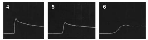
**Figure 4.** Mass velocity records of ammonals (sample 4, 5 and 6 – respectively to Table 1).
