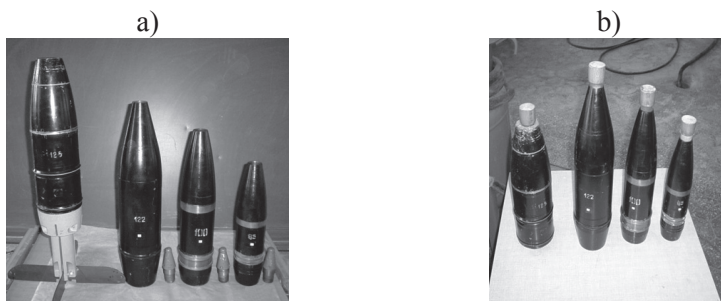
Figure 6. Examples of tested missile shells (caliber range 85-125 mm): a – shells without fuse, b – shells fulfilled with high-explosives imitator.
