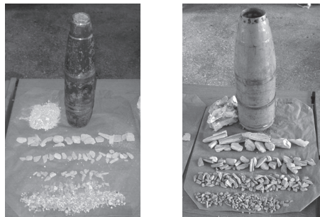
Figure 11. Typical examples of washed-out explosives fractions ( p = 40 MPa, working head equipped with two nozzles d = 0.5 mm).
