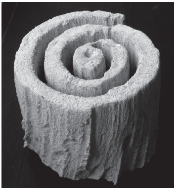
Figure 9. Examples of explosive material washed out from artillery missile ( p = 250 MPa, d = 0.7 mm).
