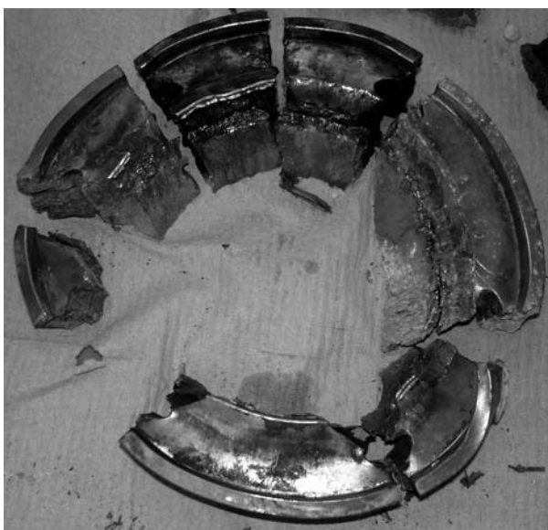
Figure 7. Showing Rear Plate fragments recovered from full detonation in target.
