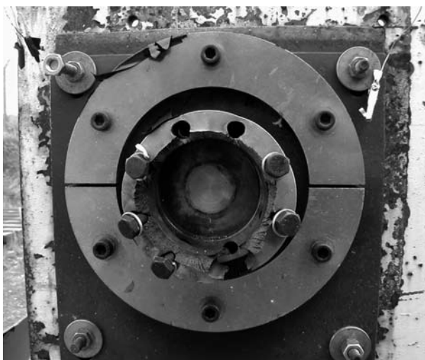
Figure 8. Firing 10 against PETN/wax showing target destruction.
