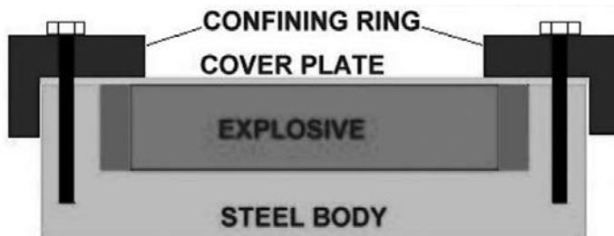
Figure 3. Modified Steven test Assembly showing increased confinement.
