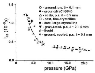
**Figure 3.** The dependence of chemical spike time  $t_{CS}$  on the pressure *P* of TNT charges detonation. p.s.  $\delta$ : explosive particle size  $\delta$ .
