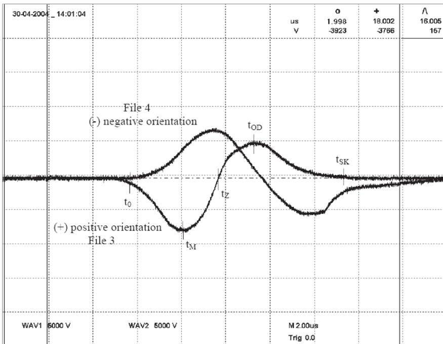
**Figure 2.** Effect of orientation of cut upon polarity of signal. Plastic explosive  $m_p = 6$  g,  $R_Z = 200 \Omega$ . File 3: Time  $t_0$  – start of pulse generating,  $t_M$  – impact of SW on free surface,  $t_Z$  – compensation of voltage,  $t_{OD}$  – impact of expansion wave front on interface epoxide – cut,  $t_{SK}$  – impact of SW on free surface.
