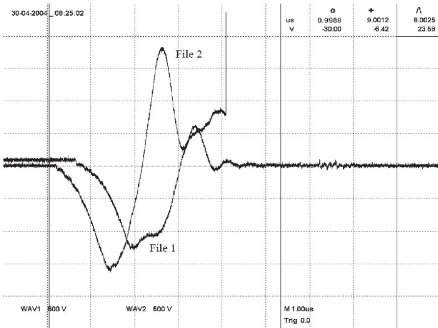
**Figure 3.** Effect of mass and type of explosive upon the signal of generator with a load of  $R_Z = 20 \Omega$ . File 1 – 4 g plastic explosive + 10 g loose explosive, File 2 – 6 g plastic explosive.
