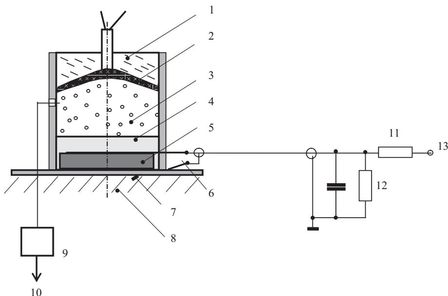
**Figure 1.** Scheme of piezogenerator: 1 – guide insert with detonator, 2 – plastic explosive, 3 – loose explosive, 4 – epoxide, 5 – piezoceramic cut, 6 – outlets from cut, 7 – cardboard or free surface, 8 – steel plate, 9 – RC switching-on circuit, 10 – external switching-on of time base of oscilloscope, 11 – high-voltage probe, 12 – generator load, 13 – input of oscilloscope.
