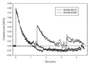
Figure 4. Overpressure profiles of incident blast waves for AN/Alp mixtures.
