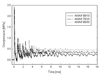
**Figure 1.** Exemplary overpressure histories recorded in the 0.15 m<sup>3</sup> chamber for ammonium nitrate/Alf mixtures.
