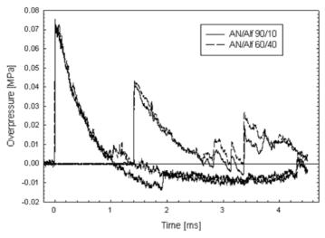
Figure 3. Overpressure profiles of incident blast waves for AN/Alf mixtures.
